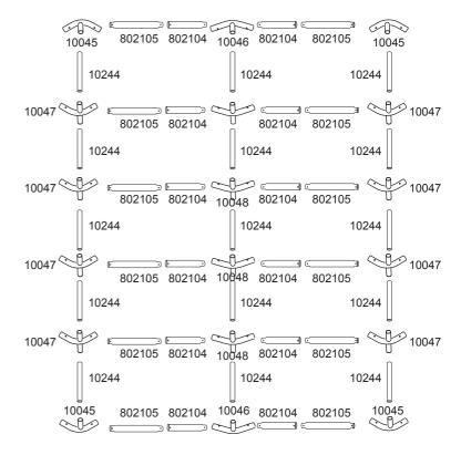
**2. Assemble Roof** Start with center, Fig. 1, using layout shown in diagram above. Bolt roof assembly together as shown in Fig. 1A. Assemble each side of the roof as shown in Fig. 2. Install #802103 truss brace roof as shown in Fig. 2A.
